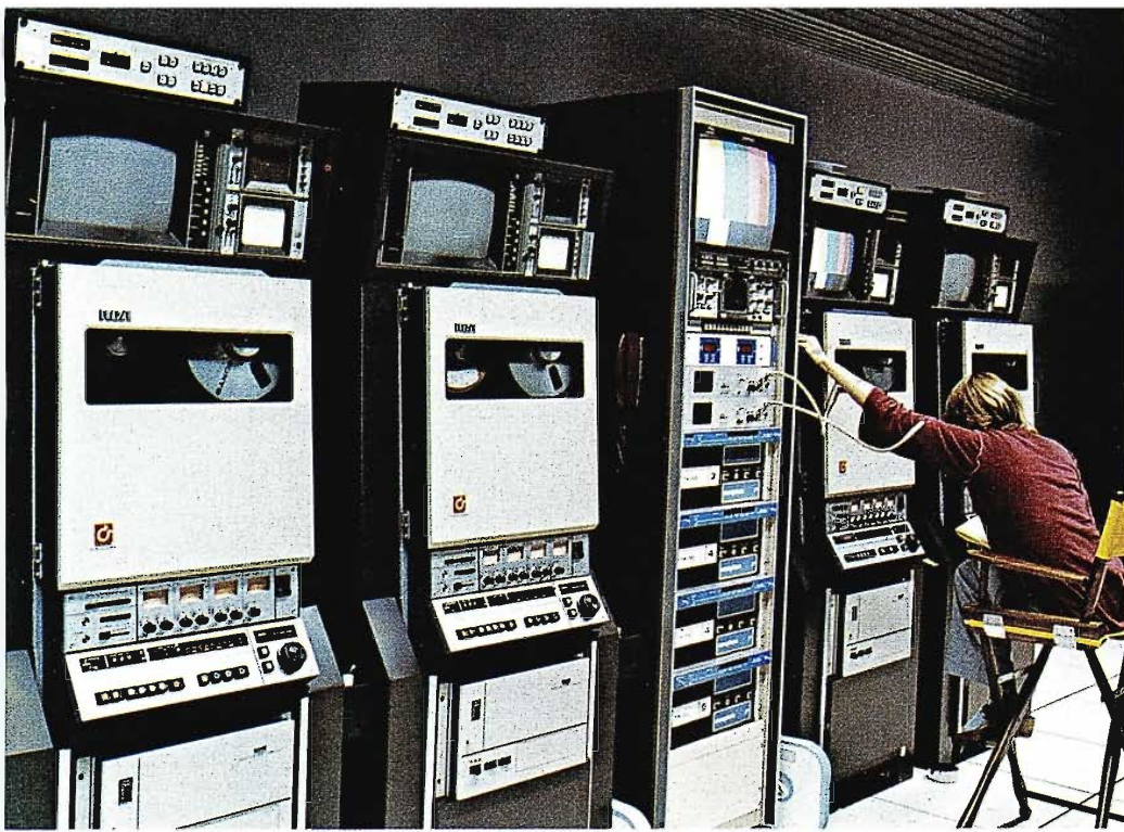
Four TH-100 one-inch VTR's in a separate group are used as auxiliary playback machines.
