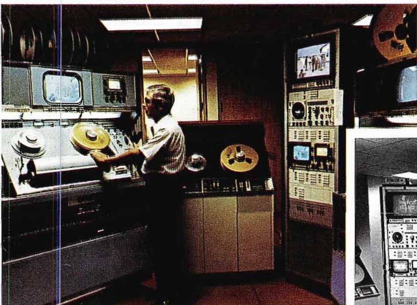
The Video Tape area at WHEC-TV features a horseshoe arrangement for operational convenience.
